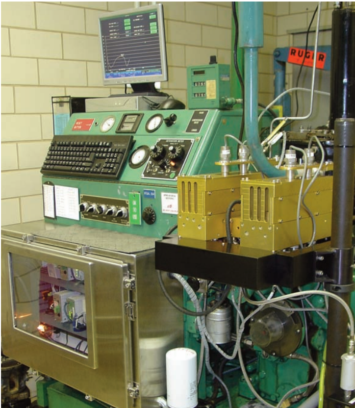
This fully automated analyzer uses multiple fuel bowls, eliminating the need to flush between determinations. Proto fuel is reduced by up to 60%, a substantial cost savings.
