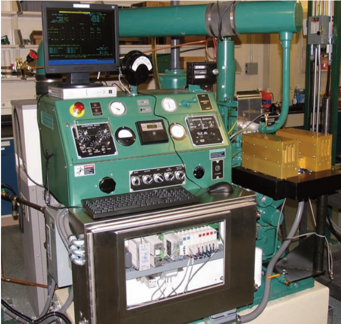
This fully automated analyzer is particularly suited for use in refineries or state, municipal, research & development or private, third party laboratories for octane number determination.
